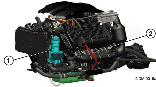
Figure 7.4 – Oil Filter and Drain
